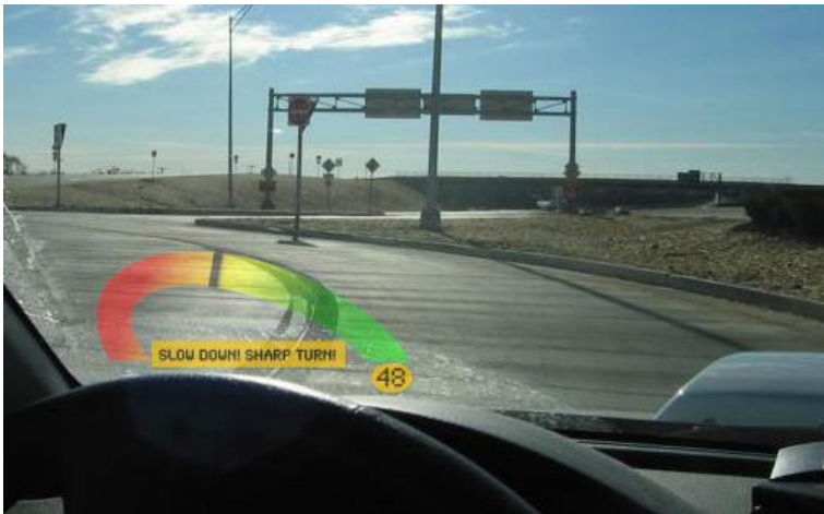
Figure 8.5: A colored dial chart shows Safety Factor and hint on the HUD. Source: Own Illustration
